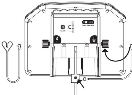
Connect the lug of the grounding cable to the grounding terminal and the prepared hole of the mounting rod.
